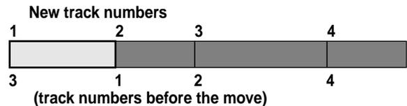
The “gap” is closed up, and all tracks are re-numbered in the new sequence. A move operation can be carried out in the stop, play ready or play modes.
